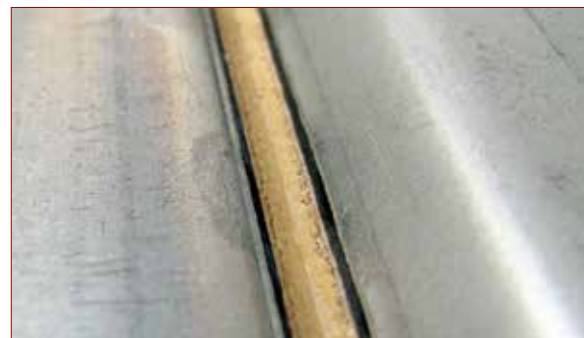
Laserline triple spot brazing result
