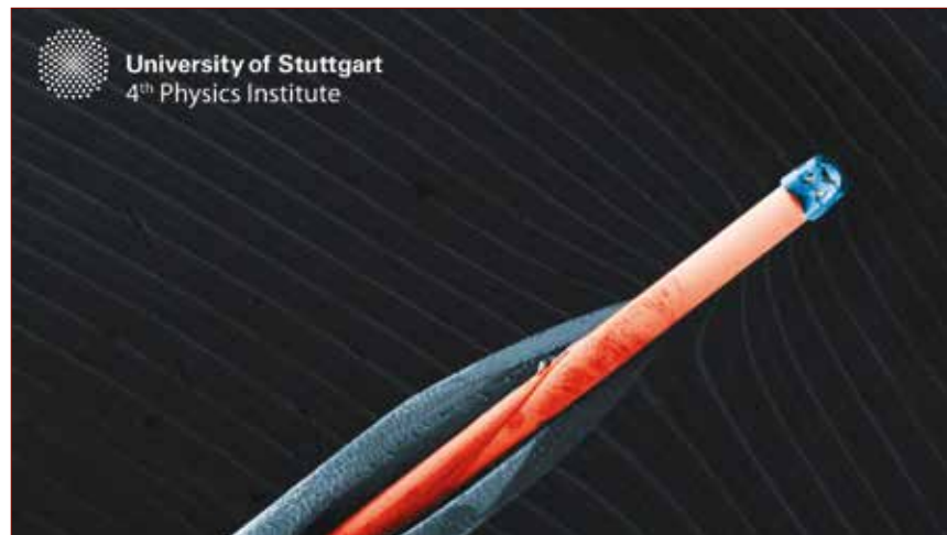
Photonics is paving the way for breakthrough innovations in medicine. Endoscopy for example uses fibre optics to get light to the point where surgery takes place and it uses fibre optics to get the image out. The next step will be devices such as this 3 lens camera with a diameter of just 125 micrometers. It has the focal length of about 3 mm and was 3D printed with a new 3D printing technology using femtosecond lasers developed by the startup Nanoscribe from Karlsruhe. Source: University of Stuttgart, 4th Physics Institute
