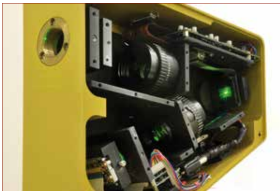
Fig. 1: The Golden Eye computational shear interferometer (without microscope objective): A liquid crystal spatial light modulator is used to encode incident light before it is imaged onto a CCD sensor. The recorded intensities are not interpretable for a human observer. However, after numerical processing, the system provides shape data with interferometric accuracy in the nanometer range and without any requirement for mechanical stabilization.
