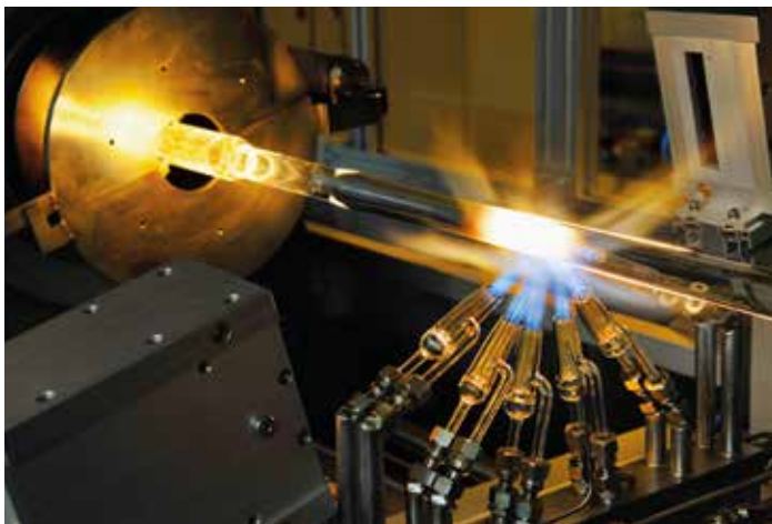
Fig. 3: Preform production for high power fiber lasers.
