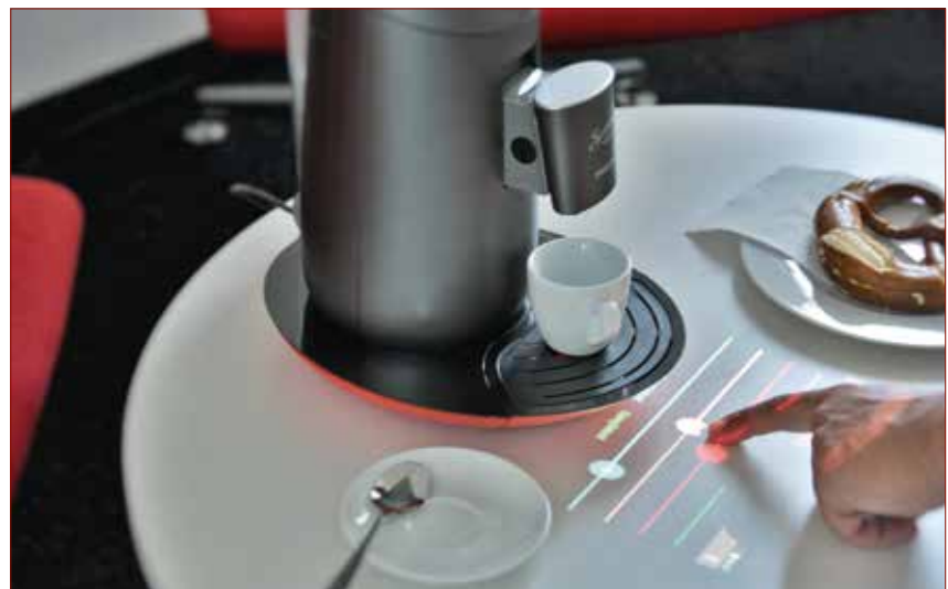
A display technology of the future will be the Picobeamer, a chip element including 3 laser diodes in the colors red, green and blue. Picobeamers will be cheap and versatile. They can project their information on any surface because of the superior depth of field of laser beamers. Connected with a sensor they will be interactive.
