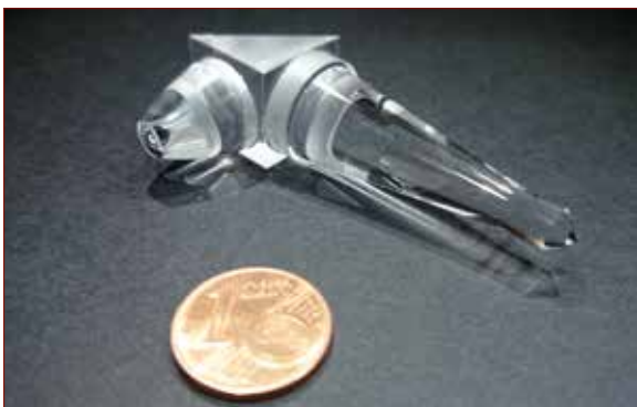
Photograph of a highly integrated system for optical tweezing (courtesy of R. Kampmann, Karlsruhe Institute of Technology/TU Ilmenau)
