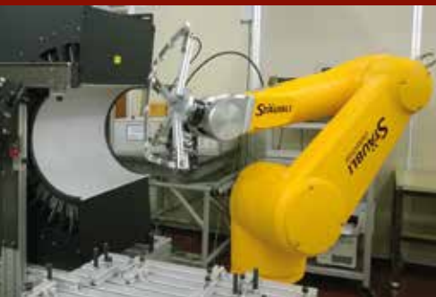
Fig 1: A robot holds the curved trim using vacuum suckers in order to move it in front of the ZEISS LineScan camera (faintly visible in the foreground on the left) on the inspection system. An elongated image of the surface is created using deflectometry technology Source: ZEISS
