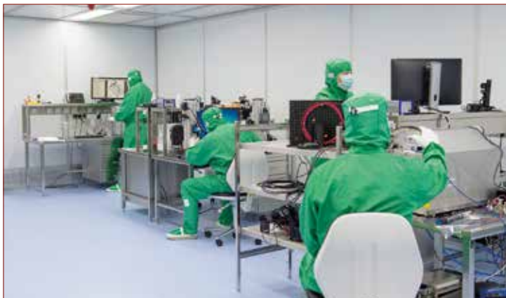
Clean room environment for the assembly of optical metrology systems (courtesy of Qioptiq Photonics GmbH & Co KG)
