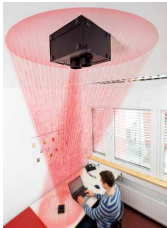
Figure 1: Li-Fi HotSpot with 1 Gbps Ethernet connectivity.
