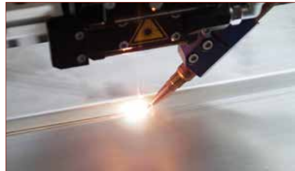
Laserline triple spot brazing process
