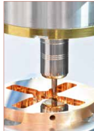
Metal optic of a particle accelerator made of copper
