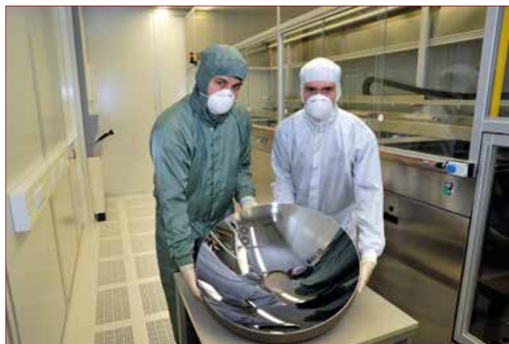
Fig. 1: Mo/Si coated EUV collector mirror for high-power LPP sources.
