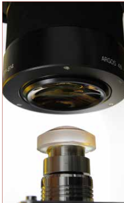
Figure 2: Testing a strong asphere on a Tilted Wave Interferometer (TWI) lab setup.
